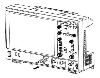
**Figure 5.3 Connecting the Passive Probe**
