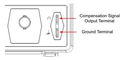
**Figure 5.4 Using the Compensation Signal**
