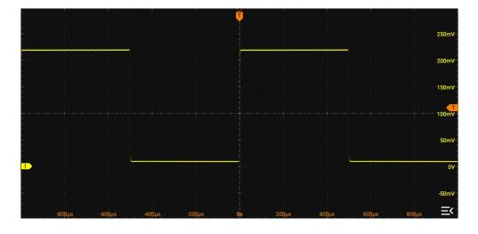
**Figure 5.5 Square Waveform Signal**
