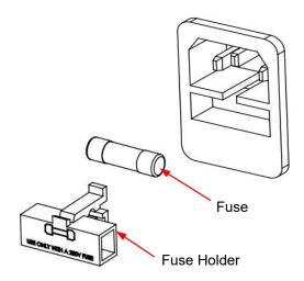
Figure 9.1 Replacing the Fuse
