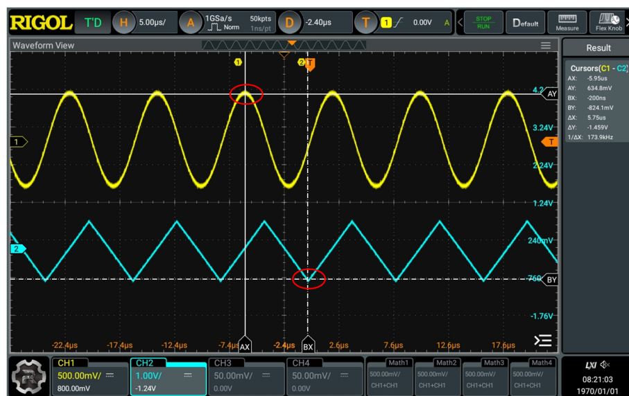
Figure 10.12 Track Measurement (before Horizontal Expansion)
