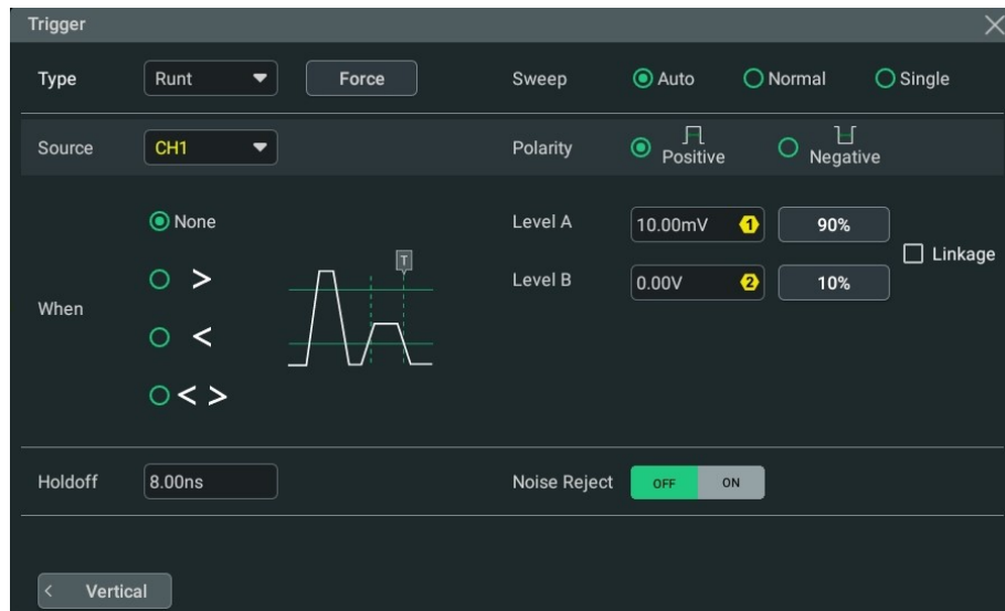
Figure 8.16 Runt Trigger Setting Menu
