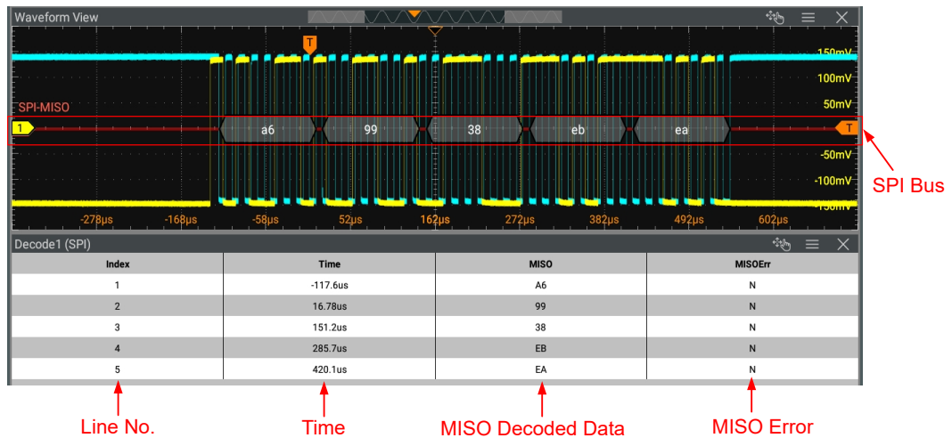
Figure 18.12 SPI Decoding Event Table
