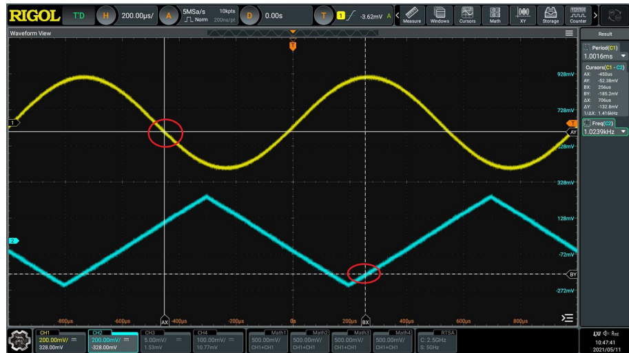
Figure 10.14 Track Measurement (after Horizontal Expansion)
